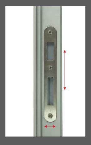
A new type of lock plate will be in use soon for most of pass doors, side doors and double wing doors. The plate is connected to the same shape plate with fixed nuts on the opposite side of door frame. After releasing screws, there is a possibility to adjust plate up/down and forward/backward in about 3 mm.
